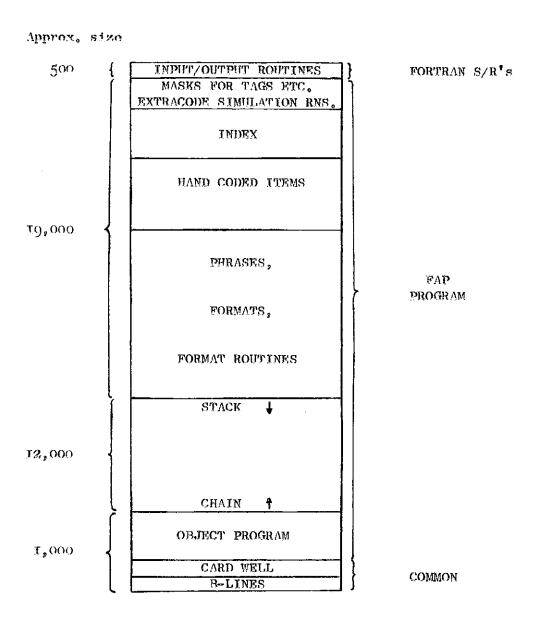
Fig 3. Storage allocation for IBM 7000 version of compiler compiler.
